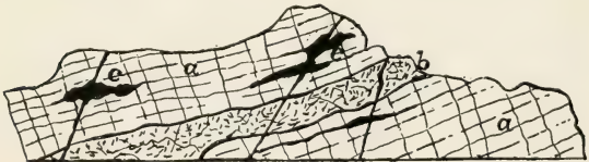
Fig. 5. Lead deposits, Derbyshire, England. After De La Beche. a.=limestone; b.=igneous rock; c.=ore.
